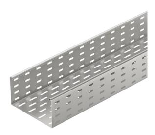
MKS 110 = medium-duty cable tray system with a side height of 110 mm. The cable tray is fastened to the bracket with screws, type FRS M6 x 12. Magnetic shield insulation without cover 20 dB, with cover 50 dB.
