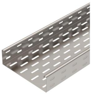
MKS 60 = Medium-duty cable tray system with a side height of 60 mm. Connecting parts should be ordered in the appropriate quantity. Magnetic shield insulation without cover 20 dB, with cover 50 dB.
