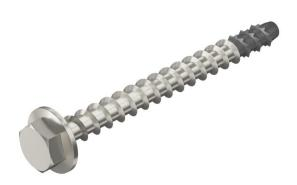
Stainless steel screw-in anchor for direct mounting without additional anchors in cracked and uncracked concrete and masonry. With hex head drive and pressed washer to accept large loads. Suitable for fastening suspended loads from suspended supports and wall brackets in wet rooms and in outdoor areas.
