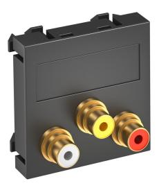
Multimedia support with three cinch connection sockets for audio/video, straight cable outlet, with labelling panel, three cinch couplings (RCA), socket-socket version, colour coding yellow/red/white. Support plate with locking fastening, suitable for horizontal and vertical installation in the system environment.
