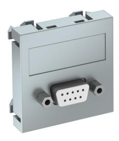
Multimedia support with one D-Sub9 connection socket, straight cable outlet, with labelling panel, D-Sub9 socket (RS232) with screw connection. Support plate with locking fastening, suitable for horizontal and vertical installation in the system environment
