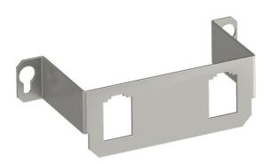
Mounting support to accept two data connection modules of the following types BTR: E-DAT; Dätwyler: MS and MS-N; Kerpen: VarioKeystone. Dimensions of a mounting opening in mm: 19.35/21.55 x 14.85. Suitable for GE2 installation unit with floor covering recess.
