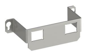
Mounting support to accept two data connection modules of the following types: Brand-Rex: shielded; EKU: E-Stone; Dätwyler: KS-T, MS-K and KU-T module; R&M: Snap-In and Keystone; Rutenbeck: UM and UMflex; SETEC: MKJ, UKJ and XKJ; Siemon TERA; Tdegärtner: AMJ and UMJ. Dimensions of a mounting opening in mm: 19.30 x 14.80. Suitable for GE2 / UDHome2 installation unit with floor covering recess. Suitable for GE2 installation unit with floor covering recess.
