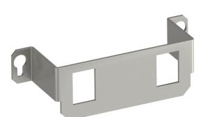
Mounting support to accept two data connection modules of the following types: AMP TYCO: Standard 110Connect, SL Series 110Connect and Toolless, AMP-Twist; Brand-Rex: unshielded; GG45; TKM RJ MOD; Nexans: LANmark with Adapter-Clip; Siemon CAT6; 3M K6 and K10. Dimensions of a mounting opening in mm: 20.10 x 14.80.
