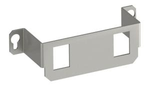
Mounting support to accept two data connection modules of the following types: AMP TYCO: Standard 110Connect, SL Series 110Connect and Tooless, AMP-Twist; Brand-Rex: unshielded; GG45; TKM RJ MOD; Nexans: LANmark with Adapter-Clip; Siemon CAT6; 3M K6 and K10. Dimensions of a mounting opening in mm: 20.10 x 14.80.
