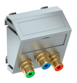
Multimedia support with three cinch connection sockets for component video, slanting cable outlet, with labelling panel, three cinch sockets (RCA) with soldered connection, colour coding red / green / blue. Support plate with locking fastening, suitable for horizontal and vertical installation in the system environment.
