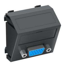
Multimedia support with one VGA connection socket, slanting cable outlet, with labelling panel, VGA socket (HD15) with screw connection. Support plate with locking fastening, suitable for horizontal and vertical installation in the system environment.
