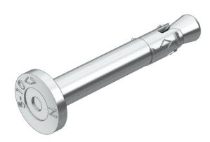
The nail anchor N-K can be used for multiple fastenings of non-load-bearing systems and in cracked and non-cracked concrete, thereby combining the benefits of a bolt tie with even easier mounting. The nail anchor only needs to be hammered into the drill hole. When the load occurs, the nail anchor spreads itself and bolts itself in the drill hole.
