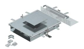
Ready-to-mount trunking extension unit with a device installation lid for the installation of an installation unit of nominal size 4, consisting of the trunking base (floor trough with side and floor covering guide profiles), trunking lid with blank mounting opening and a flushfloor end cover. The scope of delivery contains three height-adjustable wall fixing brackets, three screed anchors and trunking connection brackets.
