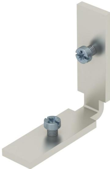
For the construction-side creation of a trunking junction as a 90° angle, T piece or crossing. A flushfloor end cover is also required for the creation of a 90° angle (order separately).
