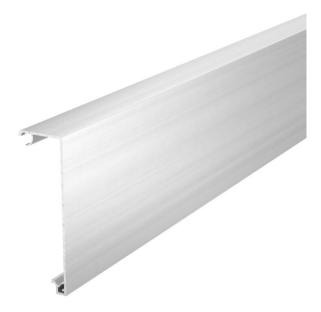
Trunking cover to create a design device installation trunking of the GAD series. "Style" design version for complete coverage of the system opening and the switching and plug-in devices. The GAD OTA cover adapters are essential and must be planned on the trunking section with a max. spacing of 50 cm. A GAD OTD spacer must be placed between the trunking covers.
