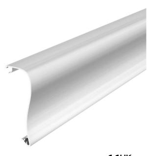
Trunking cover to create a design device installation trunking of the GAD series. "Swing" design version for complete coverage of the system opening and the switching and plug-in devices. The GAD OTA cover adapters are essential and must be planned on the trunking section with a max. spacing of 50 cm. A GAD OTD spacer must be placed between the trunking covers.
