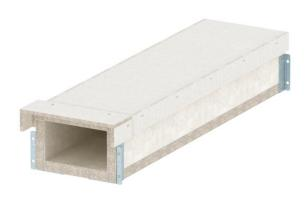
Fire protection duct made of water and frost-resistant fibreglass lightweight concrete of material class A1 according to EN 13501-1 for fireproof routing of cables in escape and rescue routes. El30 - El60 classification as installation duct according to EN 13501-2 on the basis of tests in accordance with EN 1366-5. When there is an internal fire load (cable fire), the duct prevents the spread of fire from one fire section to another.
