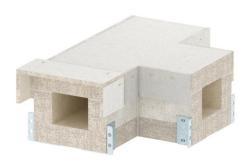
T piece for PYROLINE® Con S EI90 fire protection duct, type PLCS D090810, consisting of fibreglass light concrete which is resistant to water and frost, for the creation of T branches in the duct route. Mounted connectors ensure quick mounting in situ, whilst loosely placed covers ensure quick inspection and reassignment.
