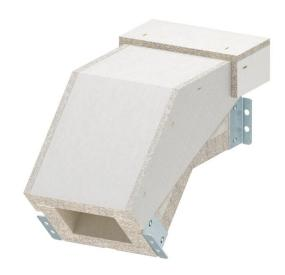
Falling vertical bend for PYROLINE® Con S El60 fire protection duct, type PLCS D060810, consisting of fibreglass light concrete which is resistant to water and frost for the creation of vertical changes of direction (45°) in the duct. Mounted connectors ensure quick mounting in situ, whilst loosely placed covers ensure quick inspection and reassignment.
