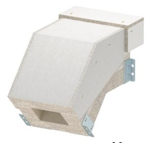
Vertical bend, falling, for PYROLINE® Con S EI90 fire protection duct, type PLCS D090810, consisting of fibreglass light concrete which is resistant to water and frost for the creation of vertical changes of direction (45°) in the duct. Mounted connectors ensure quick mounting in situ, whilst loosely placed covers ensure quick inspection and reassignment.
