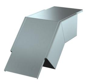
45° vertical bend, falling version, with intumescent fire protection mesh for PY-ROLINE® Rapid PLM installation duct. Suitable for direct wall and ceiling mounting, mounting below system floors and on support systems. Tool-free joint mounting with PLM SI joint connector. The cover is snapped on without tools, allowing rapid inspection and retroassignment. The cover overhang allows offset cover mounting for continuous equipotential bonding of the entire duct section.
