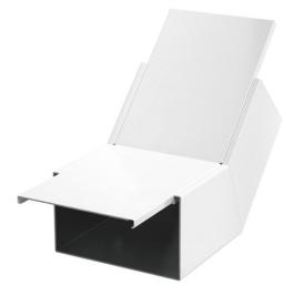
45° vertical bend, rising version, with intumescent fire protection mesh for PYRO-LINE® Rapid PLM installation duct. Suitable for direct wall and ceiling mounting, mounting below system floors and on support systems. Tool-free joint mounting with PLM SI joint connector. The cover is snapped on without tools, allowing rapid inspection and retroassignment. The cover overhang allows offset cover mounting for continuous equipotential bonding of the entire duct section.
