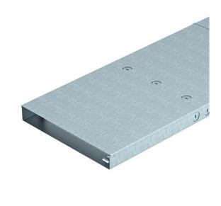
The raised floor trunking can be used for routing cables underneath raised floor panels. Retaining straps permit the self-contacting mounting of separating retainers.
