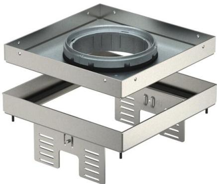
Height-adjustable cassette, decoupled from the floor, of nominal size 4, for tube bodies, for the installation of accessories in dry or wet-cleaned floors for indoor use, for mounting in underfloor boxes UZD250 or UZD350, either in conjunction with a mounting lid DUG..4 or in UGD250-3/4 or UGD350-3/4. Mounting takes place using height adjustment brackets (order separately) in the aluminium frame profile of the underfloor boxes.
