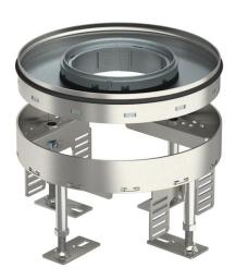
Round heavy-duty cassette for tube body of nominal size R4 for the installation of accessories in trunking systems, raised and cavity floors, in dry or wet-cleaned floors indoors. Load class 2 to 20 kN.
