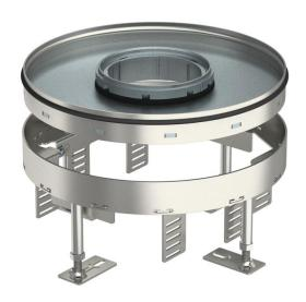
Round heavy-duty cassette for tube body of nominal size R7 for the installation of accessories in trunking systems, raised and cavity floors, in dry or wet-cleaned floors indoors. Load class 2 to 20 kN.
