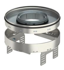
Height-adjustable cassette, decoupled from the floor, of nominal size R4, for tube bodies, for the installation of accessories in dry or wet-cleaned floors for indoor use, for mounting in underfloor boxes UZD250-3 or UZD350-3, either in conjunction with a mounting lid DUG..R4 or in UGD250-3R4 or UGD350-3R4. Mounting takes place using height adjustment brackets (order separately) in the aluminium frame profile of the underfloor boxes.
