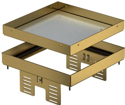
Height-adjustable "blank" cassette, decoupled from the floor, for the creation of an inspection opening of nominal size 4 in dry or wet-cleaned floors for indoor use, for mounting in underfloor boxes UZD250 or UZD350, either in conjunction with a blanking lid DUG../4 or in UGD250-3/4 or UGD350-3/4. Mounting takes place using levelling profiles (order separately) in the aluminium frame profile of the underfloor boxes. Only suitable for smooth floor coverings.
