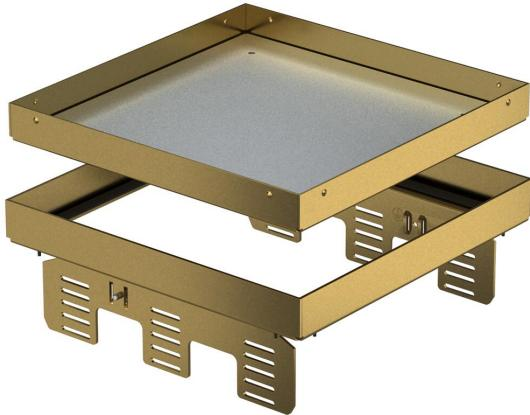
Height-adjustable "blank" cassette, decoupled from the floor, for the creation of an inspection opening of nominal size 9 in dry or wet-cleaned floors for indoor use, for mounting in underfloor boxes UZD250 or UZD350, either in conjunction with a blanking lid DUG../9 or in UGD250-3/9 or UGD350-3/9. Mounting takes place using levelling profiles (order separately) in the aluminium frame profile of the underfloor boxes. Only suitable for smooth floor coverings.
