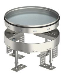
Round, "blank", heavy-duty cassette of nominal size R4 for the creation of an inspection opening in trunking systems, raised and cavity floors, in dry or wet-care floors for indoor use. Load class 2 to 20 kN. Only suitable for smooth floor coverings.
