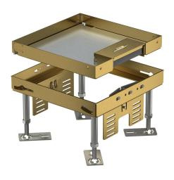
Height-adjustable cassette of nominal size 4 with cord outlet for installation of accessories in dry-care floors for indoor use. Height-adjustable cassette for cord outlet, 2-compartment. 2 APMT2 cover plates
