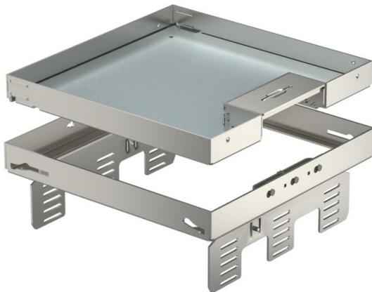
Height-adjustable cassette, decoupled from the floor, of nominal size 9, with cord outlet, for the installation of accessories in dry-cleaned floors indoors, for mounting in underfloor boxes UZD250 or UZD350, either in conjunction with a mounting cover DUG../9 or in UGD250-3/9 or UGD350-3/9. Mounting takes place using height-adjustment brackets (order separately) in the aluminium frame profile of the underfloor boxes.
