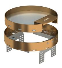
Height-adjustable cassette, decoupled from the floor, of nominal size R4, with cord outlet, for the installation of accessories in dry-cleaned floors for indoor use, for mounting in underfloor boxes UZD250-3 or UZD350-3, either in conjunction with a mounting lid DUG..R4 or in UGD250-3R4 or UGD350-3R4. Mounting takes place using height adjustment brackets (order separately) in the aluminium frame profile of the underfloor boxes.
