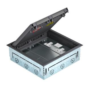
Square screed socket with GES9 UGE service outlet for use in screed floors in indoor areas. With pre-marked insertion openings for pipelines (M25) on all four sides. The delivery includes a cover plate APMT5 blank and a cover plate for 4 data connections of type LUJ6C as well as 1 cover plate APMT5 with double socket switched The minimum installation depth is 64 mm, the height-adjustment range +23 mm.
