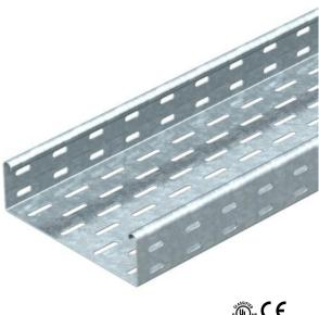
SKS 60 = Heavy-duty cable tray system with 60 mm side height. The cable tray, type SKS, should also be used for the maintenance of electrical function. For additional data, please refer to BSS fire protection systems. Magnetic shield insulation without cover 20 dB, with cover 50 dB.
