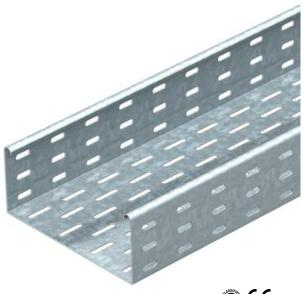
SKS 85 = heavy-duty cable tray system with 85 mm side height. FS version includes connector, type RLVL 85. Magnetic shield insulation without cover 20 dB, with cover 50 dB.
