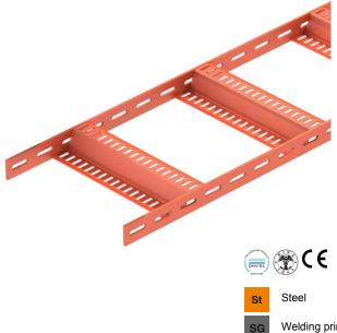
Shipbuilding cable ladder with perforated side rail of side height 40 mm with wel-ded, perforated Z rungs. Load tested according to IEC in conjunction with connector, type SLV.Welding primer type SIGMA-WELD 199, also available in white.
