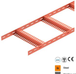
Light-duty shipbuilding cable ladder with perforated side rail of side height 35 mm with welded, perforated Z rungs. Load tested according to IEC in conjunction with connector, type SLV. Welding primer type SIGMA-WELD 199, also available in white.
