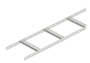
Shipbuilding cable ladder with perforated side rail of side height 25 mm with welded, perforated trapezoidal rungs which open in a downwards direction. Load tested according to IEC in conjunction with connector, type SLV. The shipbuilding cable ladder is also available in unpainted steel on request.
