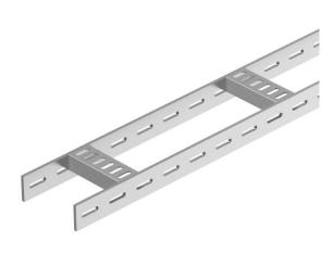
Shipbuilding cable ladder with perforated side rail of side height 40 mm with welded, perforated trapezoidal rungs which open in a downwards direction. Load tested according to IEC in conjunction with connector, type SLV.
