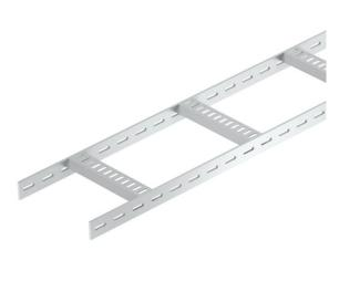
Shipbuilding cable ladder with perforated side rail of side height 40 mm with welded, perforated trapezoidal rungs which open in a downwards direction. The shipbuilding cable ladder is also available in unpainted steel on request.
