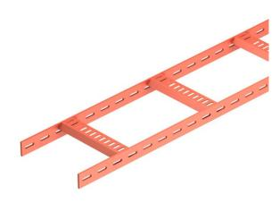
Shipbuilding cable ladder with perforated side rail of side height 40 mm with welded, perforated trapezoidal rungs which open in a downwards direction. Load tested according to IEC in conjunction with connector, type SLV. Welding primer type SIGMA-WELD 199.
