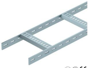
Shipbuilding cable ladder with perforated side rail of side height 40 mm with welded, perforated trapezoidal rungs which open in a downwards direction. Load tested according to IEC in conjunction with connector, type SLV. The shipbuilding cable ladder, including fittings, is also available in stainless steel on request. Powder coating according to RAL colours possible.
