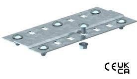
Wide joint plate for use in all cable trays and wide span cable trays. Including appropriate fastening material. For function maintenance at a width of 100 mm, the quantity of supplied M6 truss-head bolts should be increased to four, whilst for widths 200 and 300 mm, it should be increased to six.
