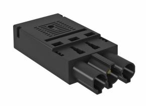
Connector part, 3-pin, type GST18i with spring power connection for rigid cables of 1.5–2.5 mm², single-wire and ultrasonically welded, fine wire cables 1.5 mm² with end sleeves, unmounted with strain relief, can be terminated in situ, 250 V, 16 A.
