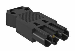
Connector part, 3-pin, type GST18i with screw connection, low height (no slot loss in combination with distributor blocks), for cross-sections of 0.75–2.5 mm², single- and fine-wire cables connectable without end sleeve, for cable diameters between 6.5–10.5 mm (H05VV, NYM), unmounted with strain relief, terminable in situ, 250 V, 16 A.
