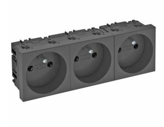
Socket with earthing pin, triple  $0^\circ$ , with increased touch protection, with screwless terminals, 2-pin, 16 A, 250 V~, with connection terminals to IEC 60884-1. For installation in Rapid 45 trunking, device installation trunking, service poles, underfloor systems and desk boxes.
