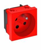
Socket with earthing pin Single 33°, encoded version, with increased touch protection, with screwless terminals, 2-pin, 16 A, 250 V~, with connection terminals to IEC 60884-1. The socket can only be used in conjunction with an encoding pin, type CST-STD.
