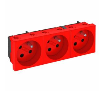
Socket with earthing pin Triple 33°, encoded version, with increased touch protection, with screwless terminals, 2-pin, 16 A, 250 V $\sim$ , with connection terminals to IEC 60884-1. The socket can only be used in conjunction with an encoding pin, type CST-STD.
