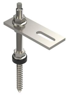
Hanger bolt set to mount photovoltaic modules on pitched roofs in combination with the TP 45 support profile. Suitable for fastening in the wooden substructure of corrugated roofs made out of plastic, tin or fibre cement. Set consists of hanger bolt with pre-mounted EPDM seal, adapter plate for the support profile and additional nuts for the optional height adjustment. Fastening of the support profile with screw with slot nut, type SKS HM (please order separately).
