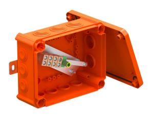
Connection box with soft plug-in seals. Sufficiently large wiring compartment through diagonally arranged connection unit with completely pre-mounted, high-temperature-resistant ceramic terminals. Green-yellow labelled protective conductor terminal. Fastening on easily accessible external flaps. Approved for cable systems that maintain the electrical function according to DIN 4102 Part 12 with the classes E30, E60 and E90. Ceramic clamps have been tested according to DIN EN 60998-2-1:2004.
